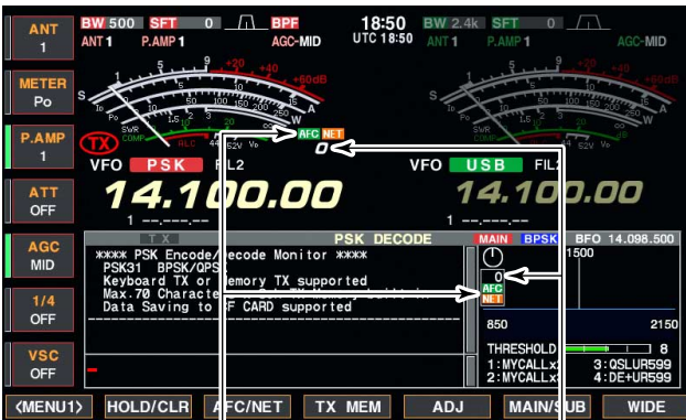
“AFC” and “NET” indicators Offset frequency
